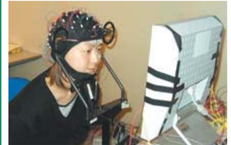
Preparation of EEG setups for BCI experiments
