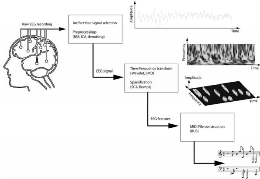
**Fig. 2.** BUS model. From EEG signals, features are extracted using a sparsification process. TF representation of the signal is obtained, and the features extracted are used to build a MIDI (“mid”) music sonification file. Illustrations on the right side are obtained from a scalp EEG record (2 sec, sampling frequency 1KHz): from top to bottom the signal, its wavelet TF representation, its bump model, and the final sonification are represented.
