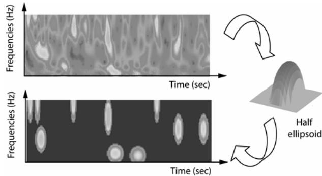
**Fig. 3.** Bump modeling, example. The TF map (*top*) is modeled by parameterized functions (*right*) into a more tractable model (*bottom*) highlighting the most prominent TF patterns.
