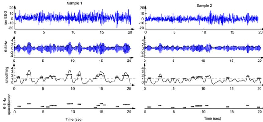
**Fig. 5.** Two examples of real-time sparsification, in the 6-8 Hz range. Top figures represent the original signal. After filtering, only the smoothed and z-score scaled activity in 6-8 Hz is analyzed (by convolution of a window of 4 time periods, here 570 msec duration). The final sparse representation (used for online BUS sonification) is displayed at the bottom.
