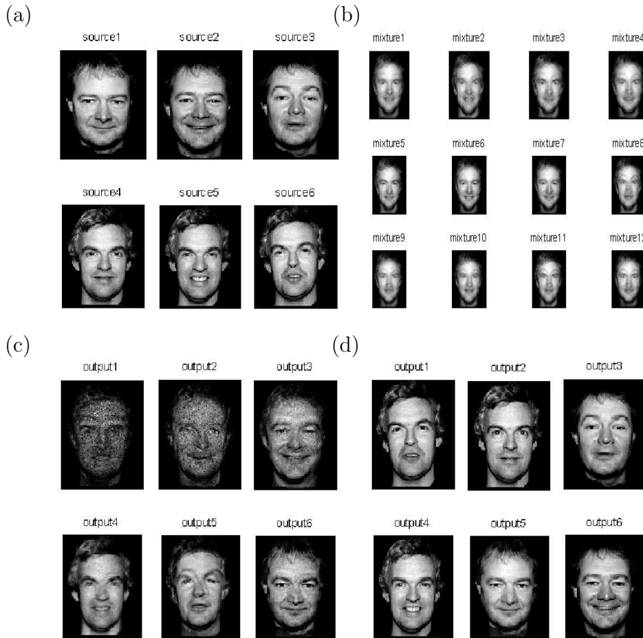
Fig. 3. Example 2: (a) Original 6 source images; (b) Observed 12 mixed images (uniformly distributed random mixing matrix); (c) Estimated source images using the standard Lee-Seung algorithm for the squared Euclidean distance (SIR = 12.1, 12.4, 13, 14.9, 12.2, 14.7 [dB], respectively); (d) Estimated source images using our QP-NMF algorithm for \lambda_A = 100 (SIR = 28.5, 35.1, 41.8, 27.2, 21.4, 34 [dB], respectively).
